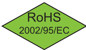
Figure 3: Example of a symbol for RoHS compliance If the printing of the RoHS symbol is not possible, marking with "RoHS" is also allowed.
